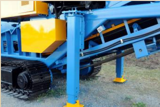
Hydraulic Leveling Legs
