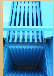
Adj. Vibrating Grizzly Feeder
