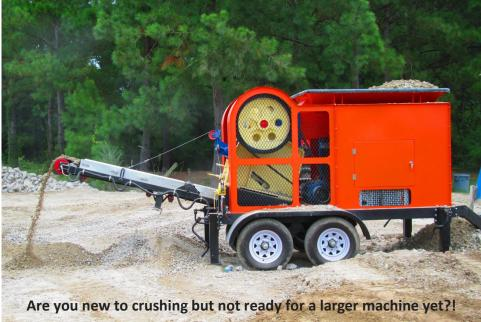
The Crushking<sup>®</sup> **Pickup Tow Crusher** is the machine for you! An ideal unit for contractors working on residential properties or in tight commercial spaces. Move this unit easily between locations and around the job site. An electric generator is installed under the feeder. The Crushking<sup>®</sup> **Pickup Tow Crusher** weighs in at approximately 10,000 lbs!
